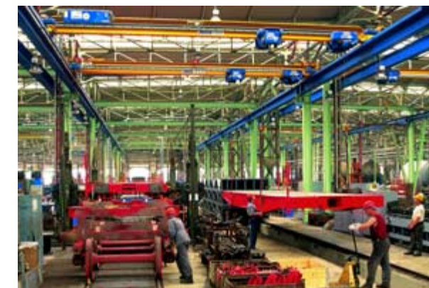
Two type E monorail hoists on type ELV single-girder overhead travelling cranes
