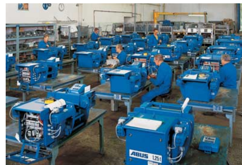
Assembly of monorail hoists
