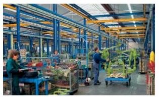
An ABUS EHB single-girder crane ensures optimum material flow on a combine harvester production line (Claas).
