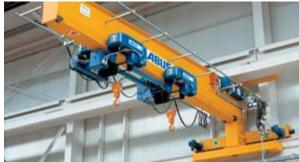
The ABUS type E electric wire rope hoist: a compact solution for single-girder travelling cranes (Rösta).
