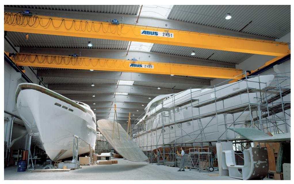
ABUS overhead travelling cranes can lift, handle and lower loads of up to 100 tonnes. Four main types are available: these include singlegirder travelling cranes, doublegirder travelling cranes for heavyduty work and wide spans and underslung travelling cranes for buildings with special conditions. The fourth main type is the wall travelling crane, installed on a separate crane track beneath the other types in order to optimise material handling.
