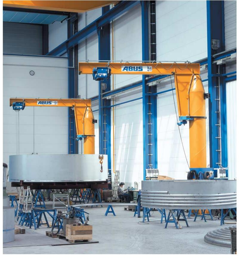
ABUS VS pillar jib crane with electric control of all crane functions used for brewing vat production (Huppmann).
