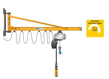
Load capacity: up to 5 t (> 4 t with ABUS wire rope hoist) Jib length: up to 10 m
