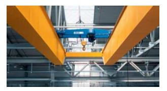
This installation benefits from the ultra low headroom design of the ABUS type DQA wire rope hoist (Bien-Haus).
