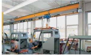
Linear point-topoint handling of vehicle cabs using the ABUS ESB monorail system (Liebherr, Ehingen)
