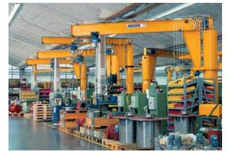
ABUS VS pillar jib crane used for assembling road milling machines (Wirtgen).
