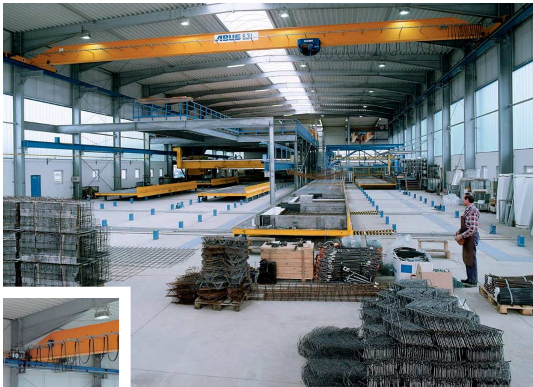
The ideal solution for a new factory: the ABUS ELK single girder travelling crane with long angle chamfer adapted to suit the building haunch (version 3), optimising available height.
