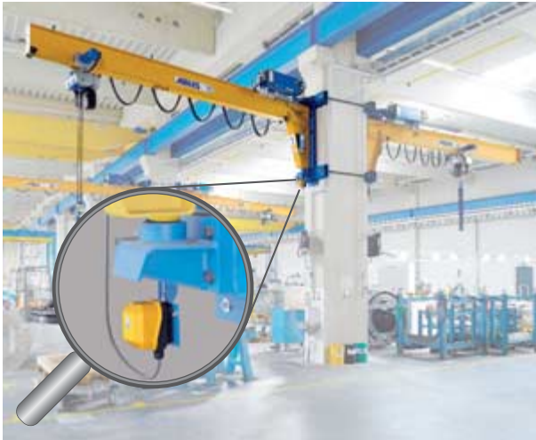
Slewing limit switch, VW (Fig. 7)
