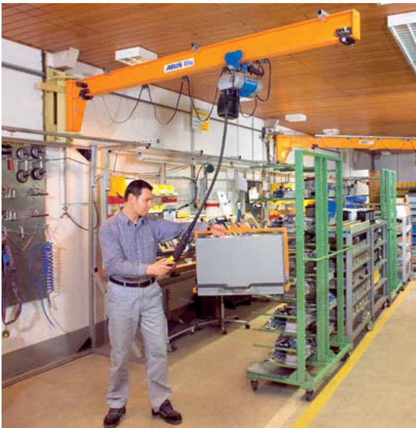
Wall jib crane LWX with electric chain hoist ABUCompact GMC
