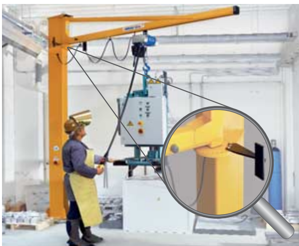
Slewing limit stops, adjustable (Fig. 5)
