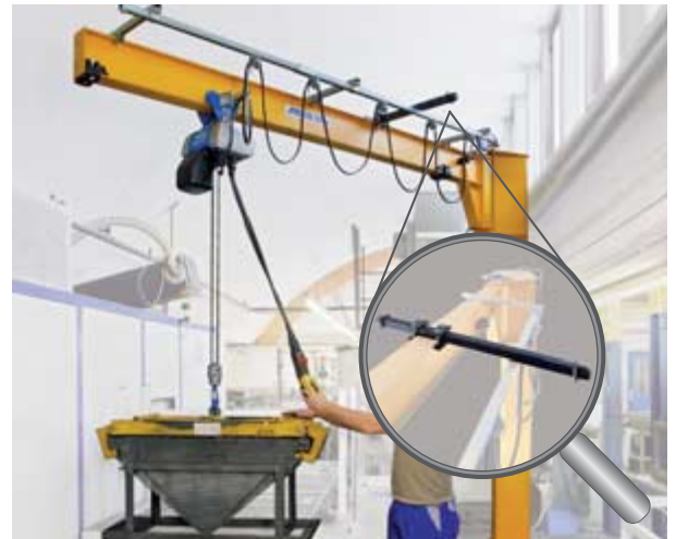
Slewing limit stop – bumper rod (Fig. 4)
