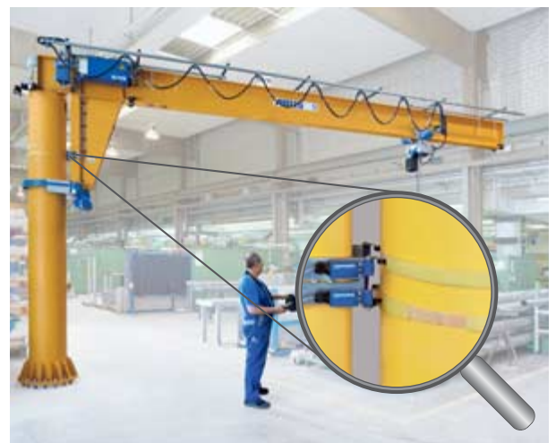
Slewing limit switch, VS (Fig. 6)
