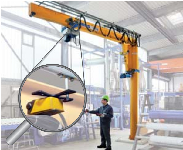
Limit switch for trolley travel (Fig. 8)
