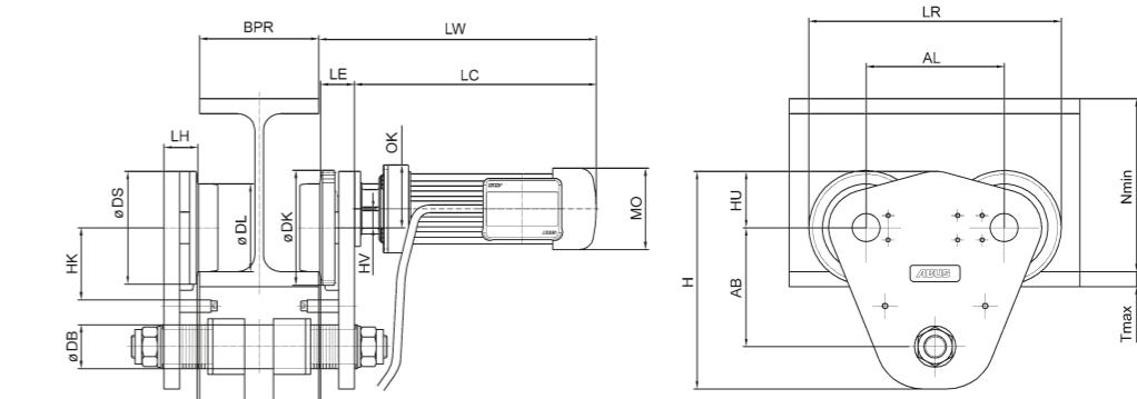
Dimension table, ABUS EF electric trolleys
