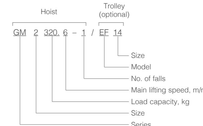
Electric chain hoists (operating voltage 230 V, 50 Hz, 1 phase)
