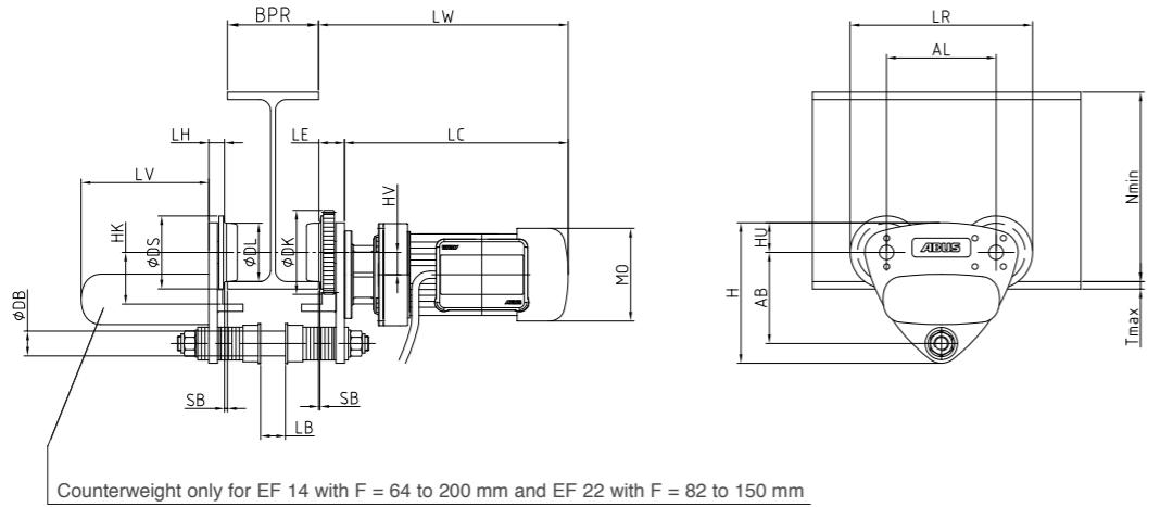
ABUS EF 50 electric trolleys
