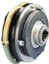
Safety brake The dual-disk electromagnetic brake features automatic braking in the event of a power failure. Asbestos-free brake linings designed for approx. 1 million braking operations make for long maintenance intervals.
