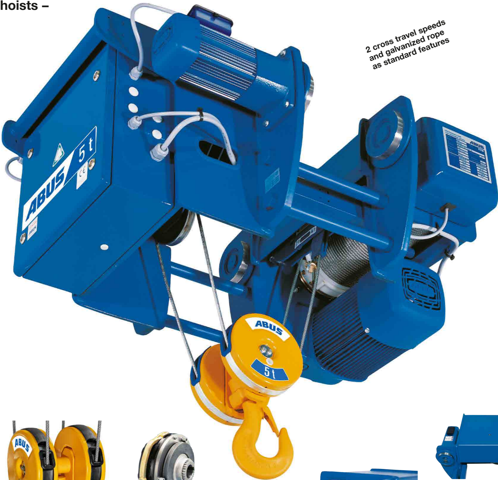
Cross travel trolley Hoist trolleys are fitted with four flanged wheels with permanently lubricated roller bearings, designed for use on tracks with parallel flanges. Wheels for tracks with inclined flanges are available as an option.
