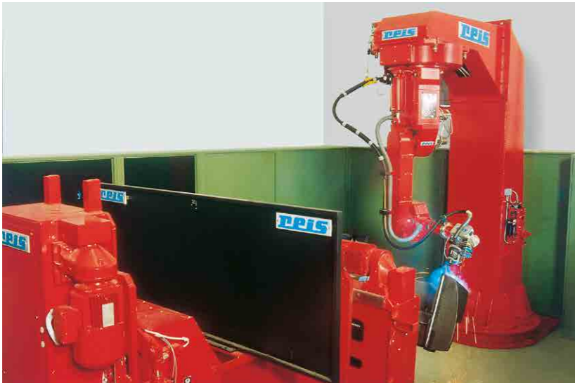
Steel trolley frames are manufactured using a 10-axis welding robot, ensuring short processing times and constantly high welding quality.
