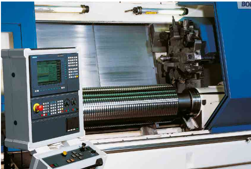
Advanced CNC lathes are used to turn the rope drums in one operation, an approach that ensures perfectly smooth running of the rope drums during operation.
