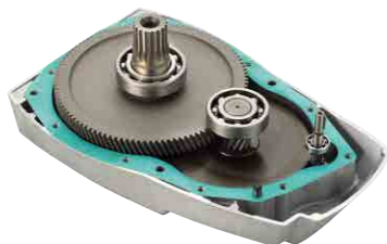
Hoisting gear Lightweight gear units with silent-running flat bevelled gears deliver the torque required. Four different gear ratios are available for each model.
